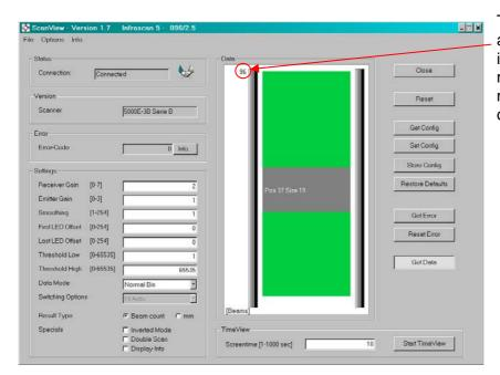
The size of the measuring area is displayed here. Either in number of beams or in mm, depending on the set output mode.
