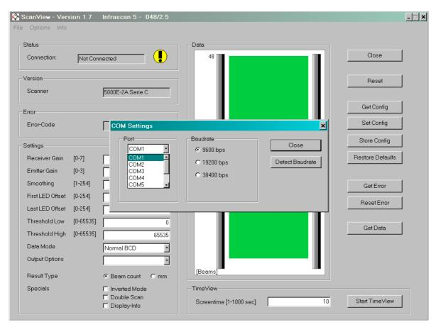
The Baud rate is not important in the first instance as the JufraScan® automatically accepts the Baud rate pre-selected by the software. You must bear in mind, however, that the latest Baud rate you selected remains stored (even after switching power off and on the scanner will use this very last stored Baud rate). In case you use a different Baud rate for communication with the scanner later on, make sure that the Baud rate of scanner and software is identical.
