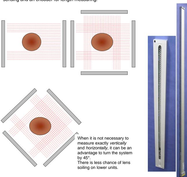
The interfaces are specially adapted for InfraScan®5000/02.5 scanners with a resolution of 1,25 mm (in the so-called Double Scan Mode) if the system is designated to be certified by the Office of Standards and Weights. In this case the use of 2 scanners for x-y-measuring is compulsory.
