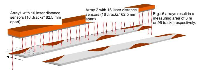
The Laser Arrays were specially developed by H-Sensortechnik. Each array combines 16 laser beams and 16 CCDs with high resolution with a powerful signal processor. By triangulation the distance to the board is being measured and thus a "profile" of the boards along the "tracks" produced.
