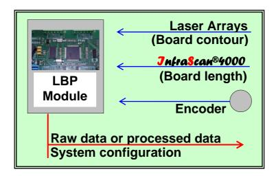
The sensor heads (laser arrays) have a nominal length of 1 m and can be "stacked" to form a system of up to 7 m length.
