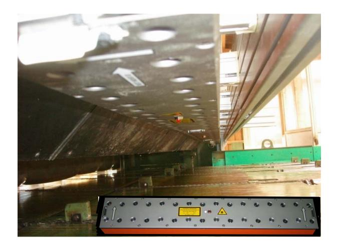
Infrared Scanning System for Measuring Wane and Dimension of Boards and Cants in Lateral Transport
