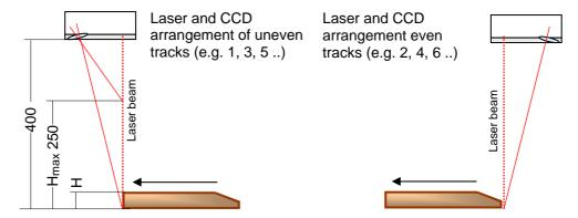
The special, alternating arrangement of the laser/CCD elements enables the system to measure very steep wane or even vertical sides very accurately.
